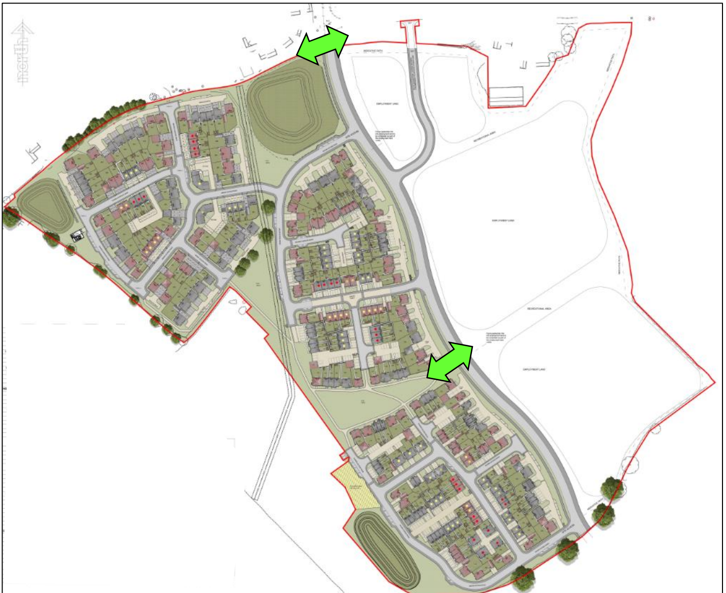
figure 21A: Preliminary crossing points [subject to s38/S278 Highways Act approvals by SCC Highways]
